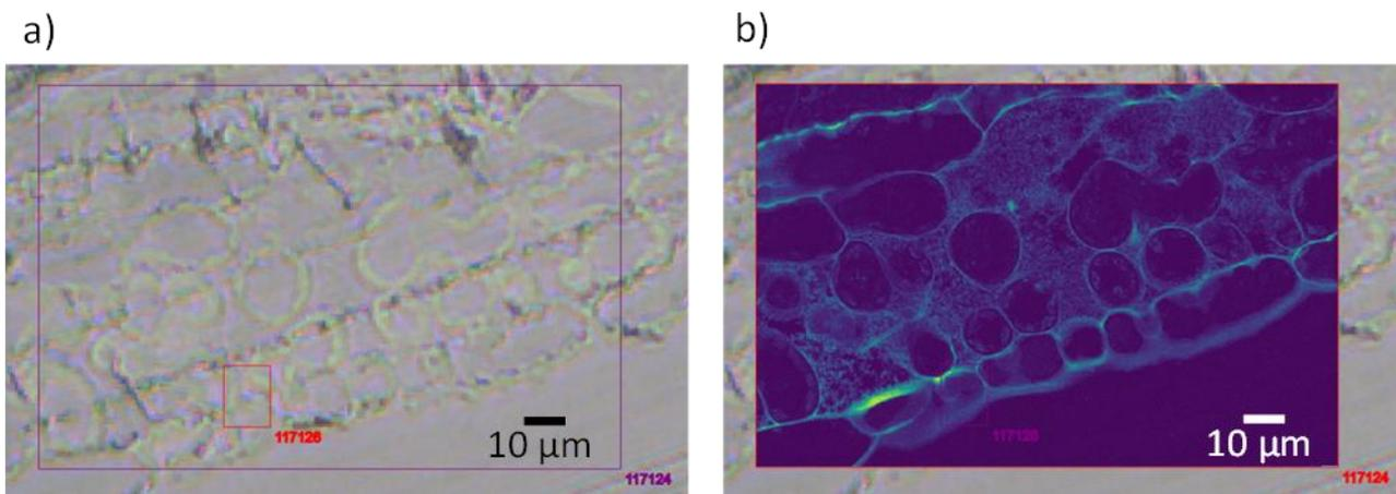
Figure 12. Overlay of Ca  $\mu$ XRF map (nano-SXM) on external OM image in bigger areas
