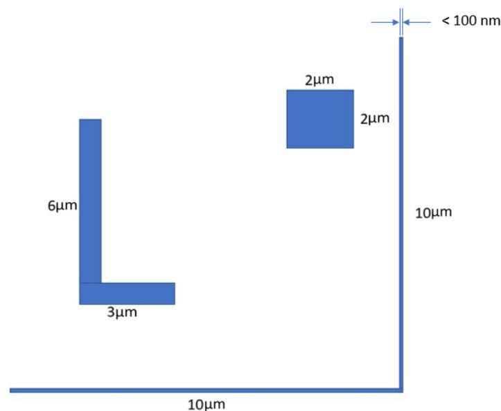
Figure 5. Pt marker design for the second membrane set
