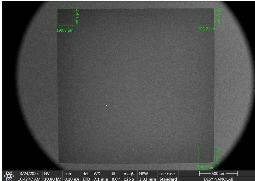
Figure 8. SEM image at 125× magnification of one  $\text{Si}_3\text{N}_4$  membrane after Pt marker deposition. The green lines show the positions of the markers in three corners. The central marker is not indicated.
