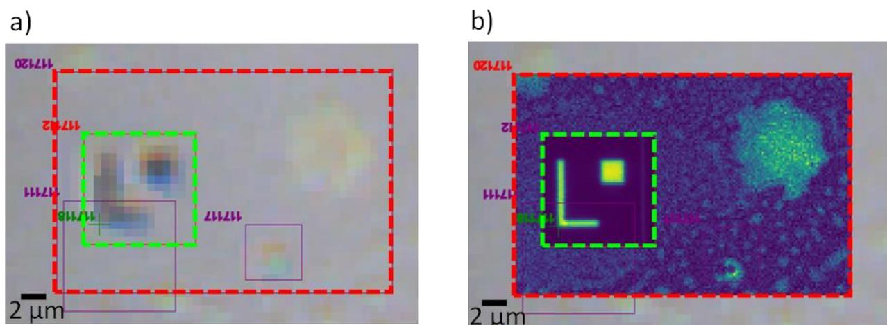
Figure 11. Verification of coordinate alignment: external OM image (a) and nano-SXM  $\mu$ XRF maps of Mn-K $\alpha$  (red) and Pt-M (green) emission (b).
