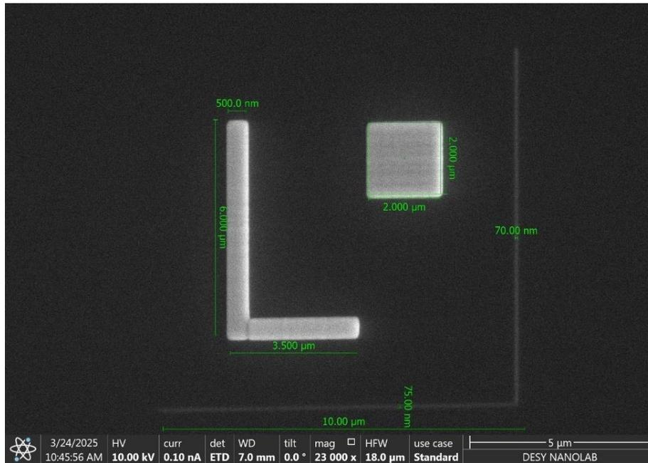
Figure 6. SEM image at 23000× magnification of one of the Pt fiducial markers deposited on one of the three membranes.
