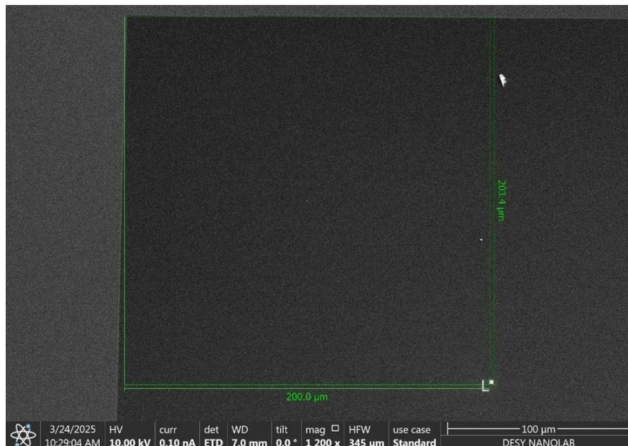
Figure 7. SEM image at 1200× magnification of the upper-left corner of one Si<sub>3</sub>N<sub>4</sub> membrane.
