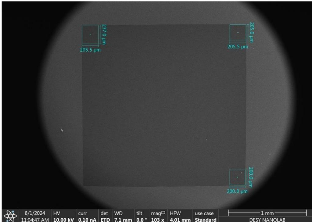
Figure 3. SEM image at 103× magnification of one Si<sub>3</sub>N<sub>4</sub> membrane after Pt marker deposition. The light blue lines indicate the positions of the markers at three corners.
