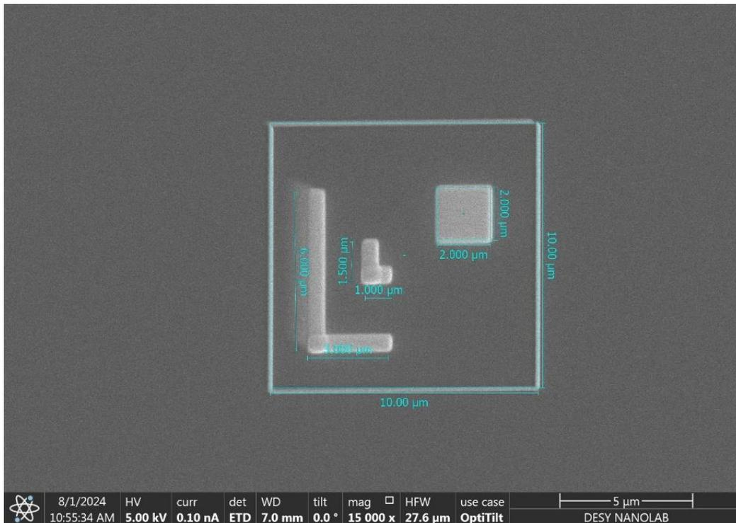
**Figure 2.** SEM image at  $15000\times$  magnification of one of the Pt fiducial markers deposited on one of the three membranes.
