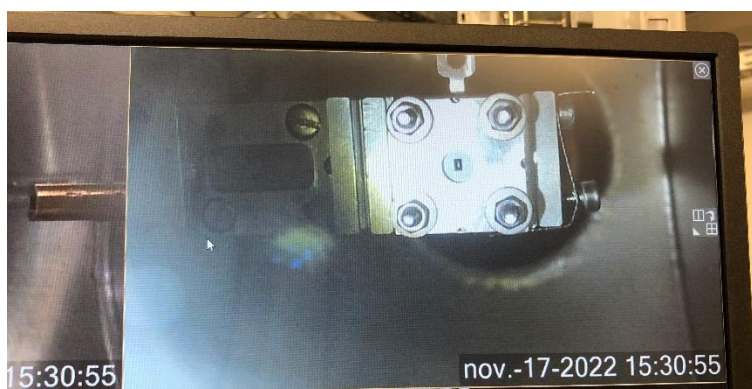
Figure 1: Picture of an assembled static liquid cell containing water in the fast-entry lock of the HAXPES endstation at the GALAXIES beamline in SOLEIL before its transfer to the analysis chamber showing the membrane (small bright rectangle in the center of the cell).
