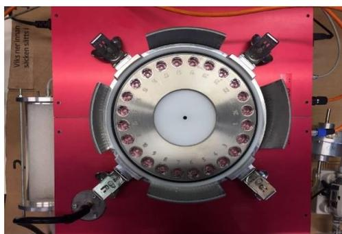
Figure 4: Nano Aerosol Chamber for In-Vitro Toxicity (NACIVT)
