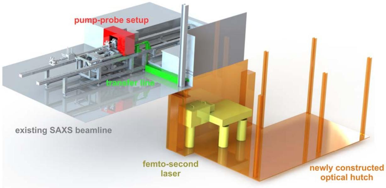
Figure 3: Overview of the beamline modifications and expansions that were made in order to accommodate the acquired femto-second laser (grey items existed prior to NFFA-Europe, coloured items were added/expanded in the framework of this project).
