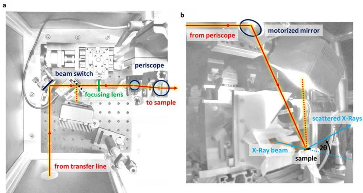
Figure 5: Laser path inside the optical enclosure module installable directly on the beamline frame. a) View of the optical components capturing and focusing the laser beam. b) Direct view of the sample stage, where X-Ray and laser beam are overlapped.
