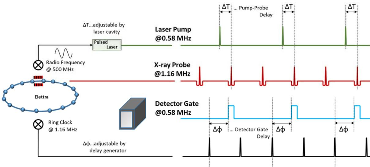
Figure 2: Timing-scheme used to synchronize the laser cavity as well as the detector gate to the timebase of the storage-ring.
