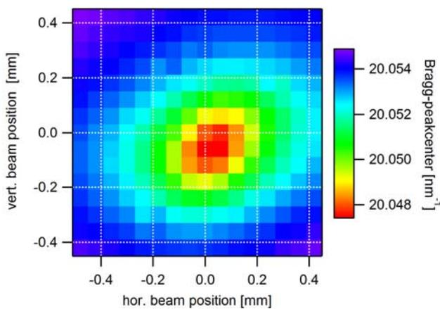
Figure 6: Spatial overlap of X-Ray and laser beam by monitoring the Bragg-peak position of the sample.
