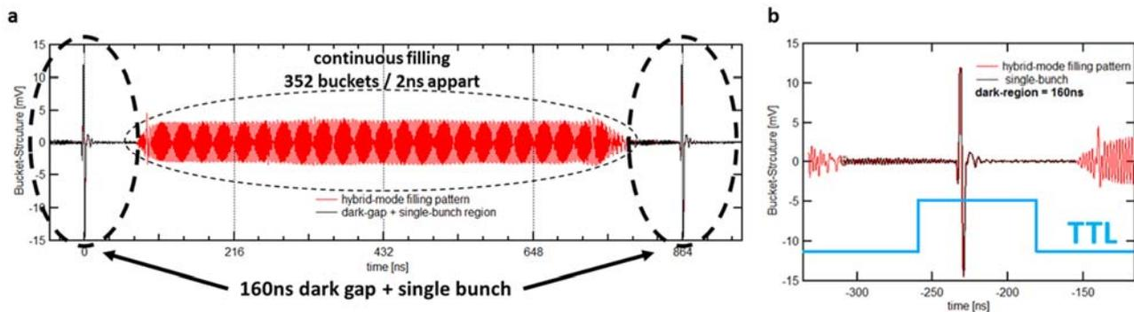
Figure 1: a) Hybrid filling mode of the Elettra storage ring, showing a “continuous filling” regime of approx. 700 ns and a single electron bunch within the 160 ns camshaft – the “dark gap”. b) Detailed view of the single-bunch in the “dark gap”, which is used as X-Ray probe for the time-resolved experiments.
