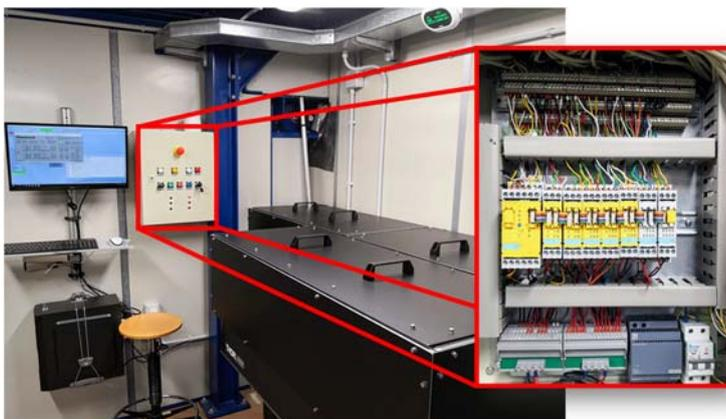
Figure 4: Photograph of the laser-head enclosure in the final laser hutch with a detailed view of the custom made PLC laser safety interlock-system.
