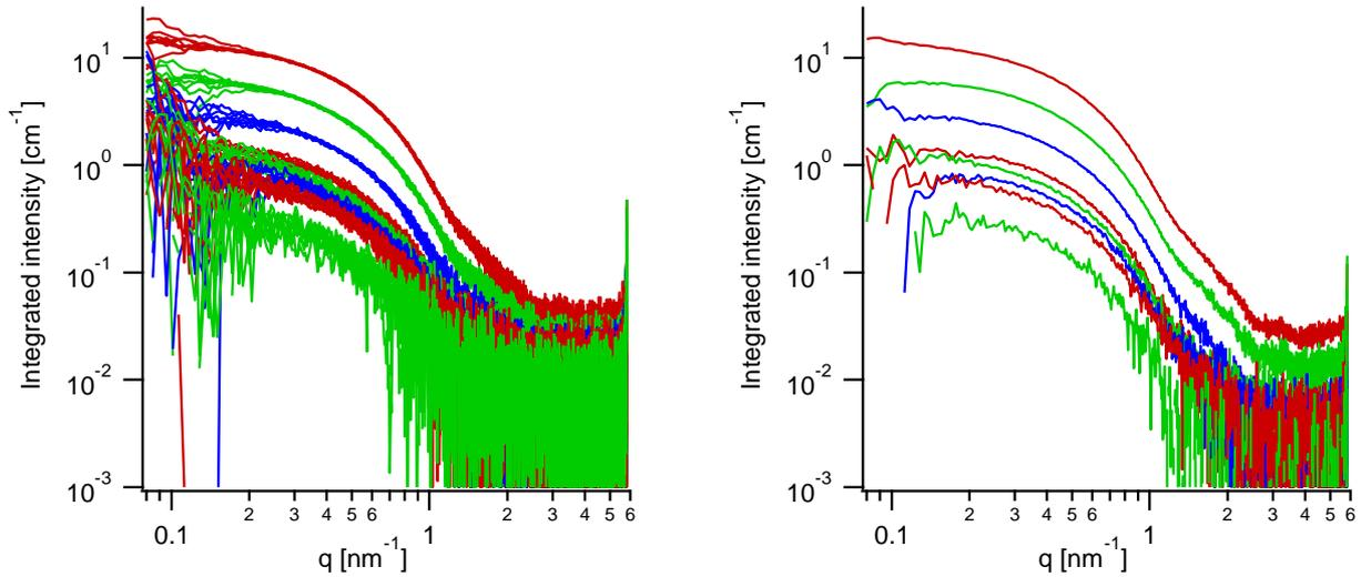
Figure 5: Scattering patterns of the BSA measurements (left) and their respective average (right). The concentrations are, top to bottom: 2.0, 1.0, 0.5, 0.3, 0.25, 0.17, 0.15 and 0.1 mg/mL.
