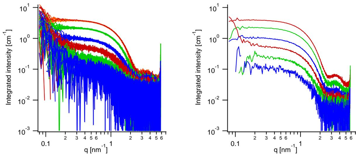
Figure 6: Scattering patterns of the lysozyme measurements (left) and their respective average (right). The concentrations are, top to bottom: 4.0, 2.4, 1.0, 0.5, 0.21 and 0.11 mg/mL.
