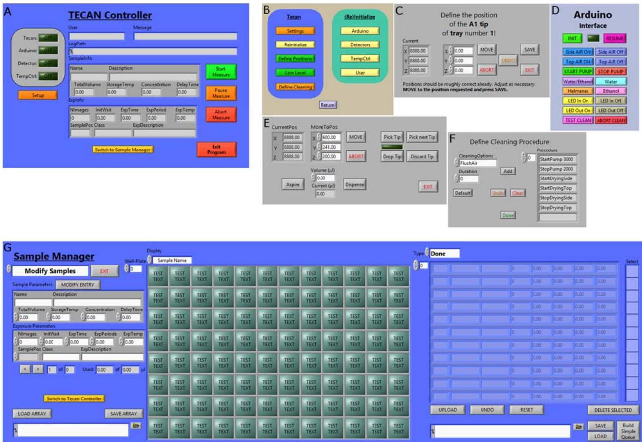
Figure 3: The different interfaces to control the sample changer. (A) The main control panel, (B) the selection window for the various sub programs, (C) the alignment assistant, (D) the low-level panel for the Arduino board controlling pump and valves, (E) the low-level control of the robotic arm, (F) the cleaning procedure creation assistant and (G) the sample manager.
