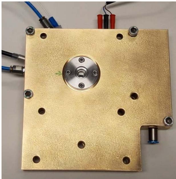
Figure 2: The final prototype cell made from brass. One of the cylinders holding the silicon-nitride windows is seen in the centre. Connections are visible for (clockwise from the left) the first drying air stream, the camera for internal imaging, the cleaning fluids, the second drying air, the power for the internal lighting and the connection for the waste drain tube.
