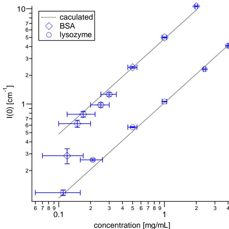
Figure 7: The measured, absolute forward intensities,  $I(0)$ , of the different concentrations of both proteins, plotted against their concentration measured with UV-vis. The dotted lines are the expected values calculated from the absolute scattering in the forward direction,  $I(0)$ , given in [9].
