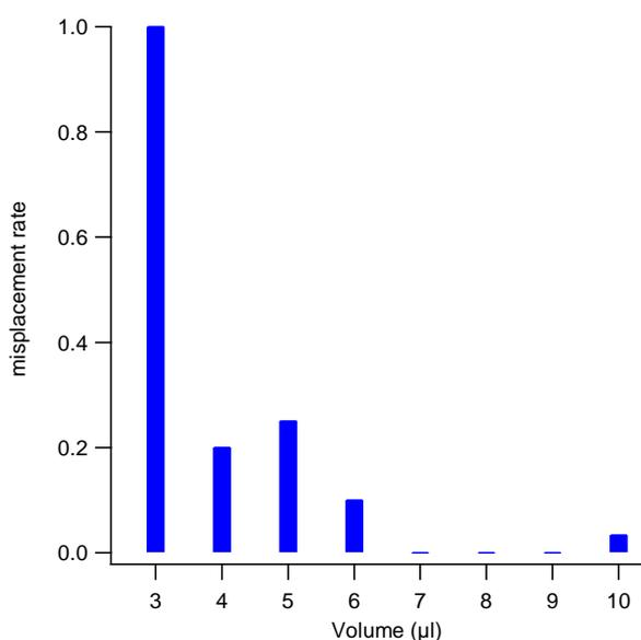
Figure 4: Misplacement rate (misplaced drops/number of tries) for different volumes at a window distance of 0.6 mm. At volumes below 7  $\mu\text{L}$  drops often don't cover the whole window anymore. At 3  $\mu\text{L}$  the volume is too low even to be placed between the windows.
