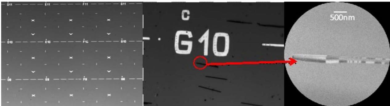
Figure 4: Optical light microscopic images of dedicated markers with close-by nano regions of interest obtained from a soft X-ray beamline at SOLEIL (R. Belkhou, CNRS / SOLEIL).
