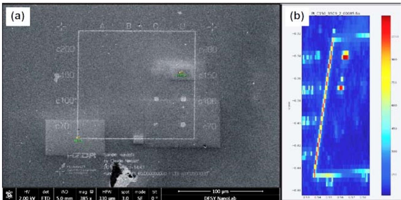
Figure 2: SEM image (left) and Pt X-ray fluorescence image (right) of electron-beam lithography prepared Pt nano-arrays with surrounding localization frames and marker numbers (S. Kulkarni, T. F. Keller, R. Shayduk, A. Stierle et. al, DESY)
