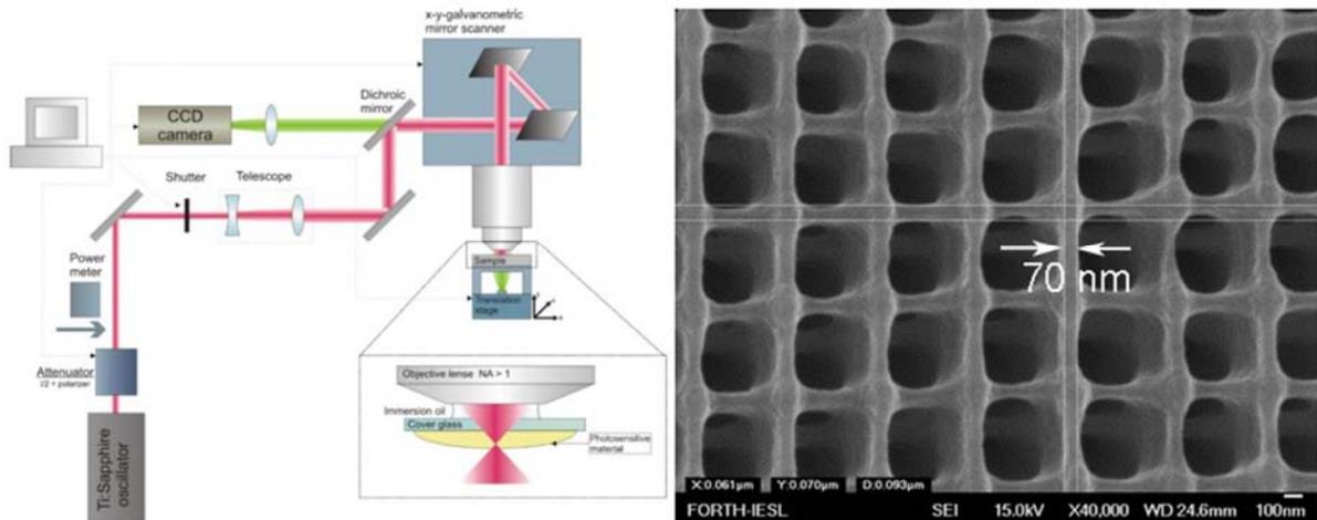
Direct laser writing via multiphoton polymerization workstation at **FORTH**
