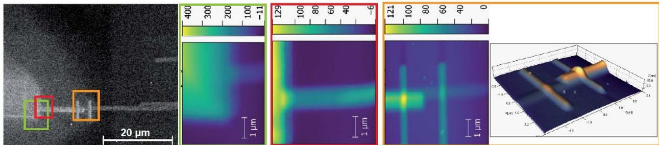
Figure 3: SEM, 2D- and 3D-AFM images of the EBID/IBID written Pt based markers during the navigation to the pre-selected nano-object (E. Graanaes, S Kulkarni, M. Abuin, T. F. Keller, A. Stierle, DESY).
