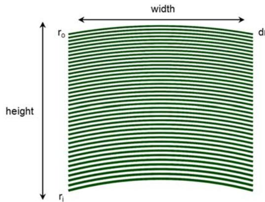
Figure 3 – Scheme of an off-axis zone plate, with its most important parameters indicated: the outer radius ( $r_o$ ) corresponds to the half diameter of the Fresnel zone plate the off-axis part is cut out, the inner radius ( $r_i$ ) determines the number of the innermost zone, and the area is determined by the height and the width of the optical element, whereas the height is the difference of  $r_o$  and  $r_i$ .  $dr$  is the line width of the outermost opaque zone.
