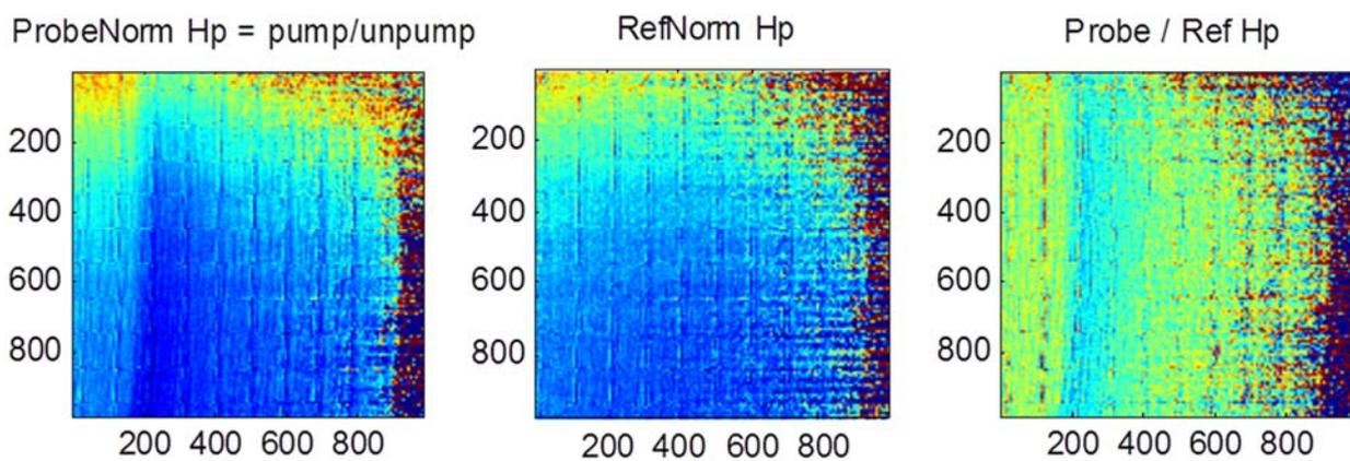
Figure 8 – Demagnetization of a permalloy film. Left: Image on the probe CCD camera. Middle: Image from the reference camera. Right: Divided image, showing the transmission change. The scale is in pixels; each pixel has a time delay of 28 fs, giving a whole time window of 2.6 ps. The time delay increases from left to right.
