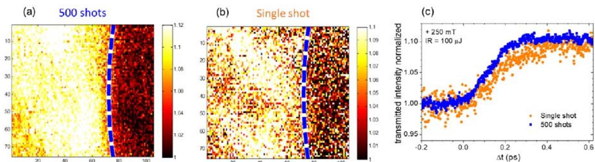
Figure 6 – XMCD signal change in transmission upon pumping a magnetic film with an IR laser. (a) Average image of 500 shots, (b) similar detector image for one single shot, and (c) time-dependent transmission change as averaged perpendicular to the time-dispersive direction as indicated with the blue line in (a) and (b).
