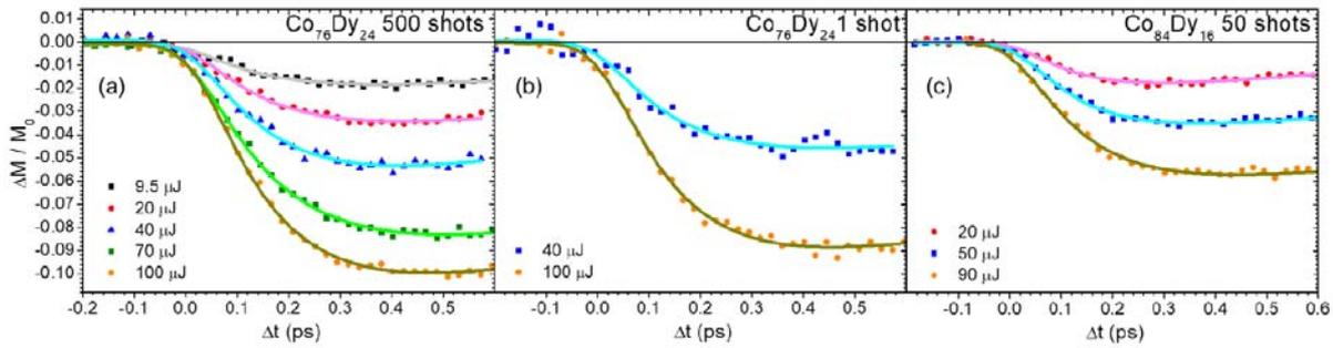
Figure 7 – Demagnetization dynamics of different alloys und different pump fluences. (a)  $\text{Co}_{76}\text{Dy}_{24}$ , 500 shots, 9.5 – 100  $\mu\text{J}$  pulse energy; (b)  $\text{Co}_{76}\text{Dy}_{24}$ , 1 shot, 40 and 100  $\mu\text{J}$  pulse energy; (c)  $\text{Co}_{84}\text{Dy}_{16}$ , 50 shots, 20, 50 and 90  $\mu\text{J}$  pulse energy.
