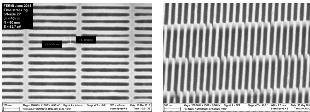
Figure 4 – SEM images of the zone plate structures. Left: 40 nm wide lines directly patterned from HSQ. Right: 40 nm wide structures etched 180 nm deep into a 340 nm silicon membrane.
