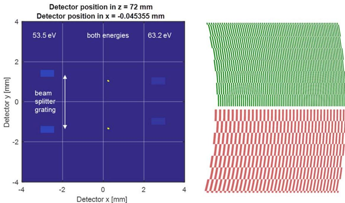
Figure 5 – Combined off-axis zone plate and beam splitter grating for two different energies (right). Left: the calculated detector image shows the traces of the EUV radiation in the focal plane when the optical element is irradiated with two light of two colours in a pre-defined energy ratio.
