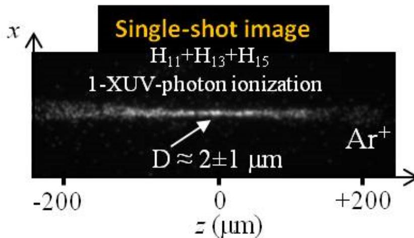
**Figure 4.** Single-shot ion distribution recorded at the focus of an XUV beam which contains the harmonics from 11th to 15th. The ion distribution was produced through 1-XUV-photon ionization of argon. From. ref. [13].
