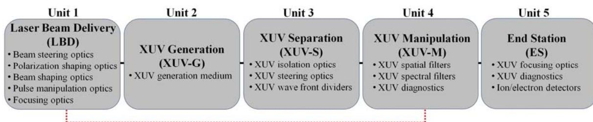
Figure 1. Block diagram of XUV beam lines. From Ref. [1]
