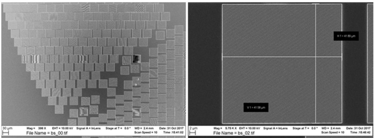
Figure 2: *SEM images of a condenser for Zernike phase contrast microscopy.* The left hand side shows a part of the condenser on its left side. Periodicity and line orientation of each field is calculated in a way that all fields diffract to the same field of view. The right hand side shows a zoom-in on one of the fields.
