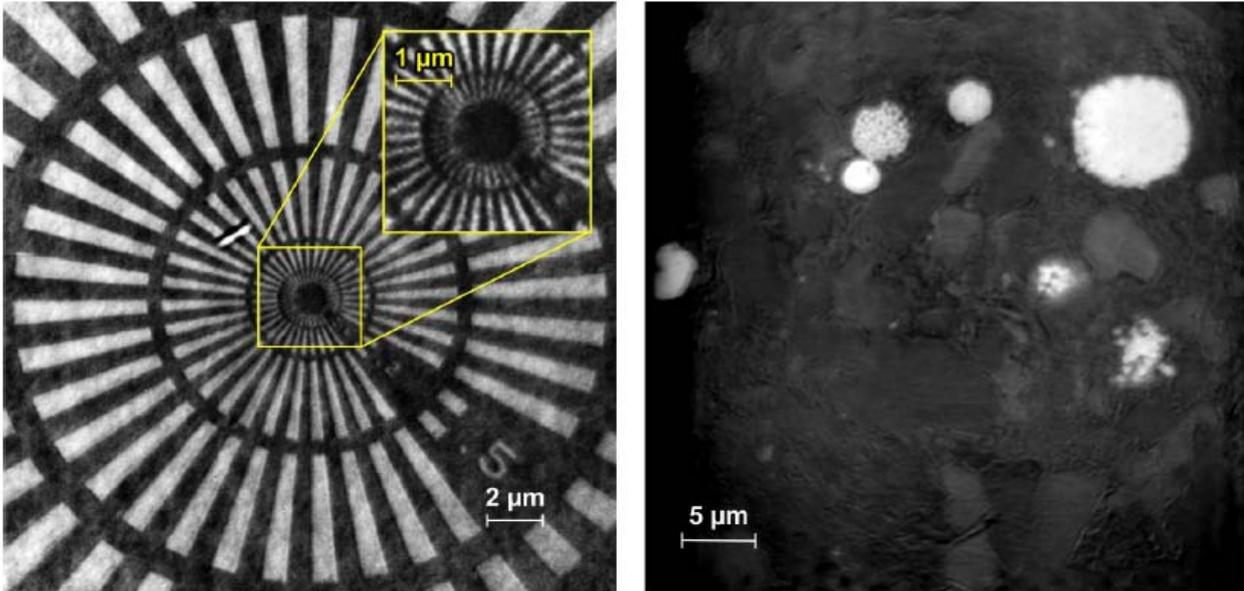
Figure 4: *Transmission X-ray micrographs recorded using the Zernike full-field setup.* left, Detail of a micrograph that shows a reference sample with smallest lines and spaces of 50 nm (centre of inset). right, Sagittal slice of local tomography on a shale-rock sample with pyrite inclusions (light gray). The sample had a diameter of 160  $\mu\text{m}$ .
