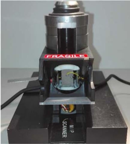
Figure 2: Image of the N9524A scanner used in the set up
