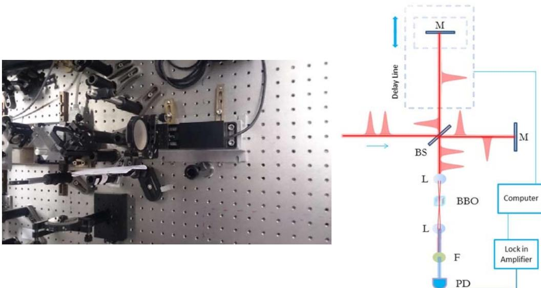
Figure 1: Left side: Picture showing the Michelson interferometer in the laboratory. Right side: schematic Michelson-type interferometer. BS: Beam Splitter, M: mirror, L: lens, F: low-pass filter, PD: photodiode.
