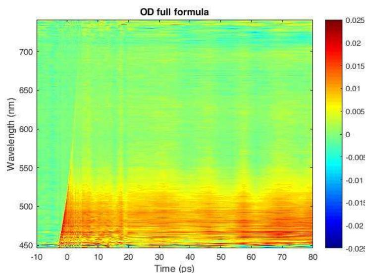
Figure 5. A time- & wavelength-resolved measurement of a thin film of a metal oxide as a result of the pump-probe workstation operation. Horizontal and vertical cross sections will reveal the ultrafast electron dynamics of the system.
