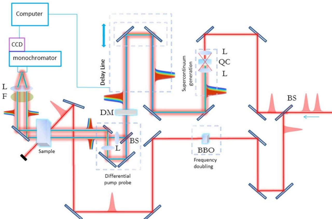
Figure 3: Differential pump probe setup. BS: Beam Splitter, L: lens, DM: dichroic mirror, F:band-pass & absorbance filters. The initial pulse pair and the generated supercontinuum pulses appear spatially separated for representation purposes.
