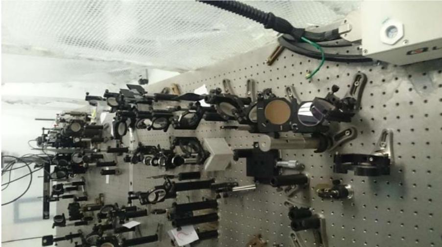
Figure 6. The optics comprising the Non Collinear Optical Parametric Amplifier.
