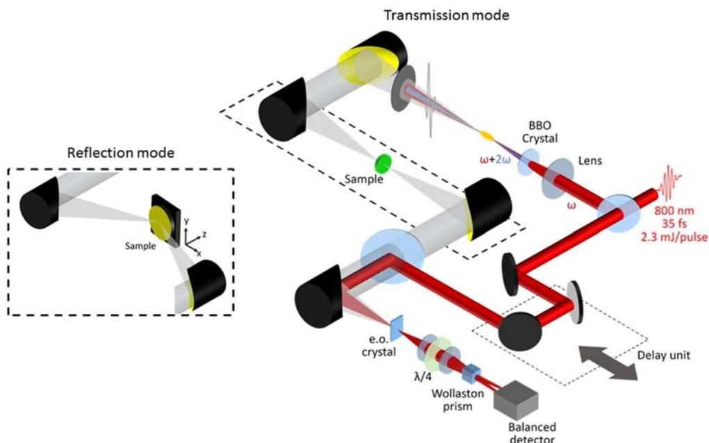
Figure 7. Terahertz time-domain spectroscopic (THz - TDS) setup.
