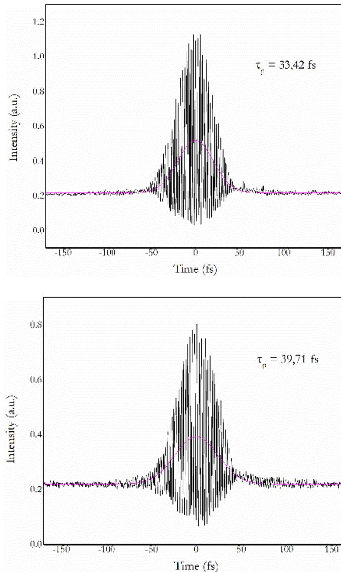
Figure 2: Temporal autocorrelation. above: almost fully compressed pulse, below: not optimally compressed (chirped laser pulse).
